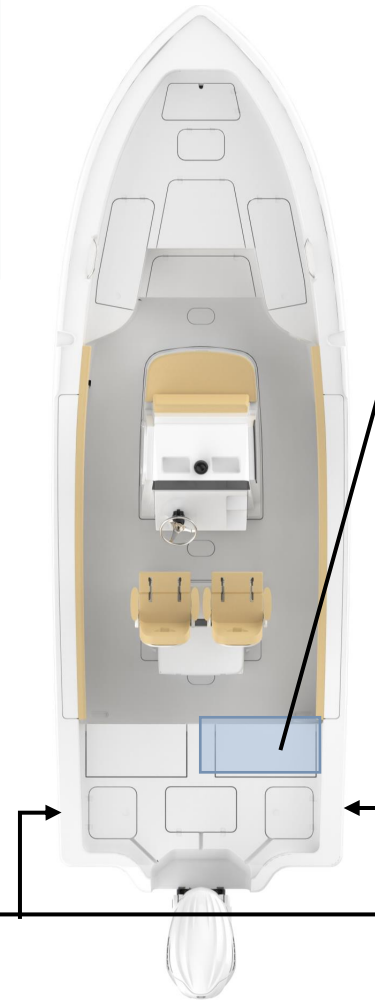
The rear seat easily opens to allow easy access to the bilge area at the stern.
